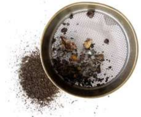
Figure 7. Additional testing performed with a 2mm sieve.
