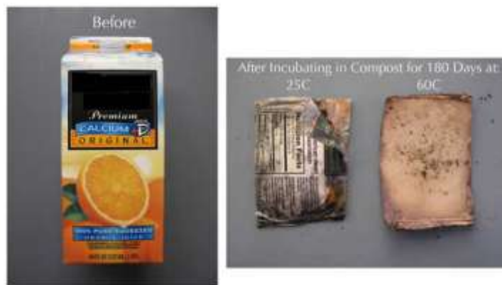
Figure 5. Before and after photos of a plastic-coated paper juice carton show the plastic coating separating from the paperboard.
